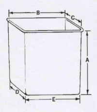
A is measured from the bottom of the rim to the base of the insert. B & C measurements are taken one inch down from beneath the lip, on the outside of the insert.
