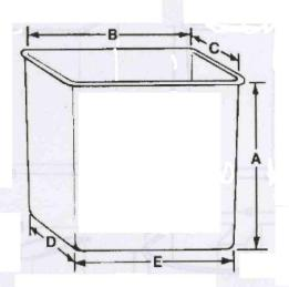
D & E measurements are taken three inches up from the bottom, on the outside of the insert. This eliminates distortion due to the radius of the corners.
