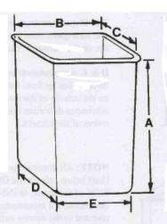
A is measured from the bottom of the rim to the base of the insert. B & C measurements are taken one inch down from beneath the lip, on the outside of the insert.
