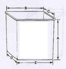
A is measured from the bottom of the rim to the base of the insert. B & C measurements are taken one inch down from beneath the lip, on the outside of the insert.
