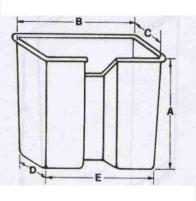
NOTE: All dimensions shown in chart below refer to the OUT-SIDE of the insert, or INSIDE of the bucket. All measurements are rounded to the nearest half-inch.
