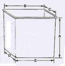
D & E measurements are taken three inches up from the bottom, on the outside of the insert. This eliminates distortion due to the radius of the corners.
