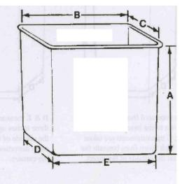
A is measured from the bottom of the rim to the base of the insert. B & C measurements are taken one inch down from beneath the lip, on the outside of the insert.
